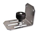
Adjusts for doors from 5/16" to 3-5/8". Mounting holes countersunk to protect door finish. 8-gauge zinc plated stel with black 2" diameter non-marring roller.
