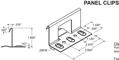
STANDARD CLIP: for U.S. rated and engineered solid deck applications. Accommodates for unlimited thermal movement in both directions. Clips are fabricated from Grade 50 G90 base steel, 18 ga.
