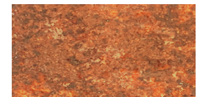
Rusteel Plus™ (A606) potential look after weather exposure
