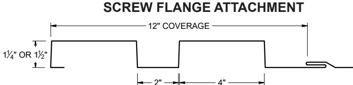
Screw Flange panels in this profile require additional material (drop/waste) and must be slit to a custom size. Inquire for custom pricing and availability.
