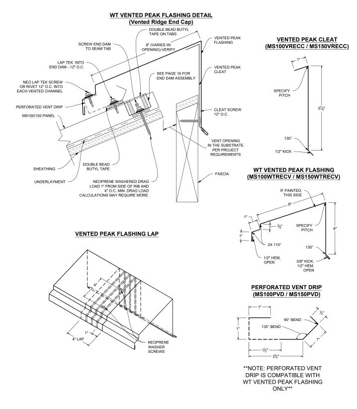
**Note:** All screws must be fastened into solid substrate. Flashing must be lapped 4" with 3 rows of gunnable sealant. **Pitch Change**
