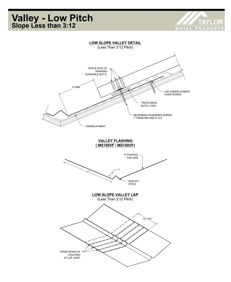
Note: All screws must be fastened into solid substrate.
