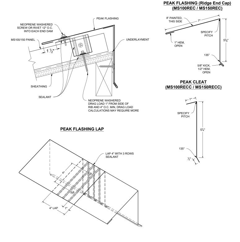
**Note:** All screws must be fastened into solid substrate. Flashing must be lapped 4" with 3 rows of gunnable sealant.
