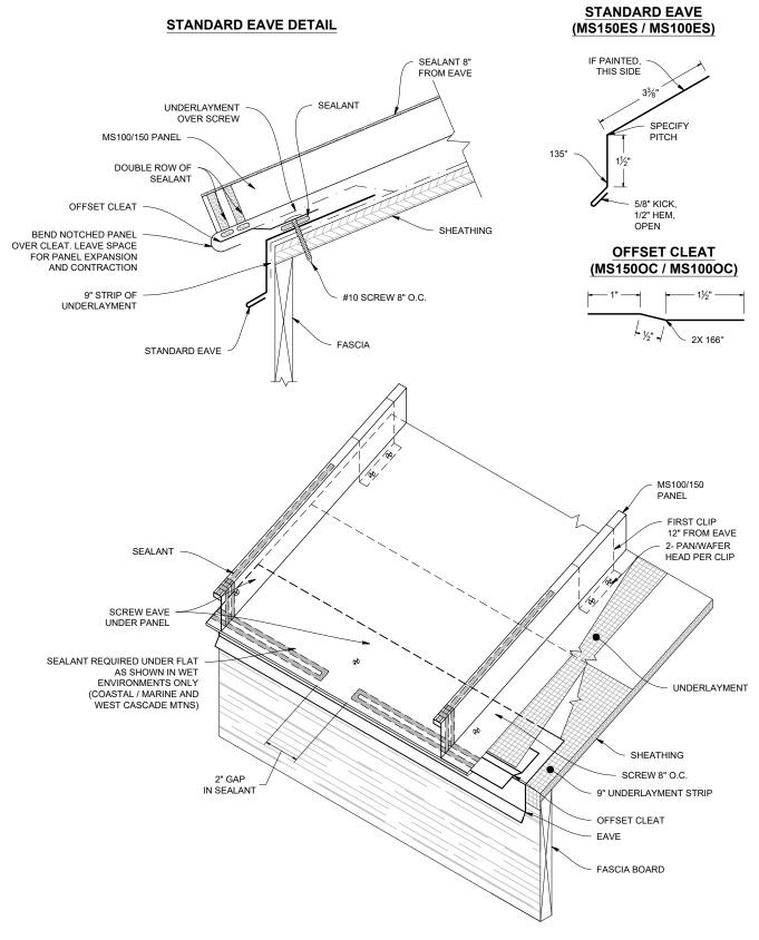
**Note:** All screws must be fastened into solid substrate. Flashing must be lapped 4" with 3 rows of gunnable sealant.
