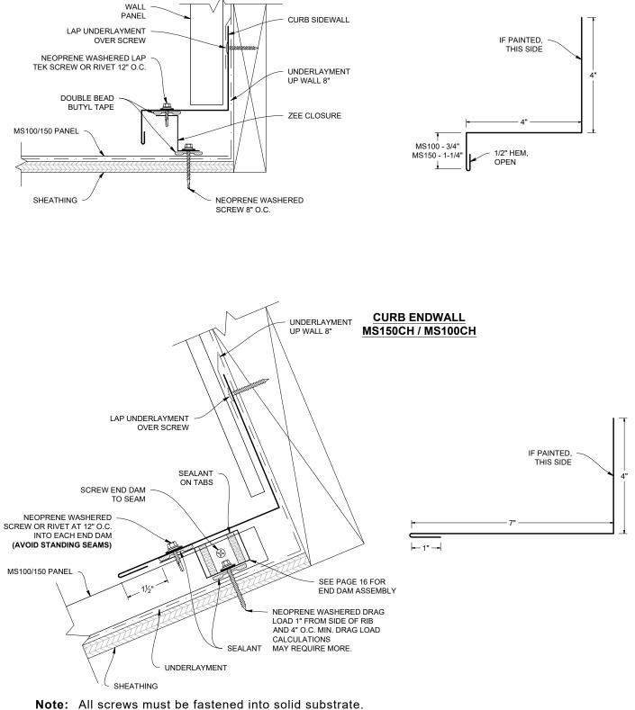
Flashing must be lapped 4" with 3 rows of gunnable butyl caulk.
