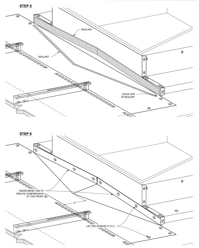
Note: All screws must be fastened into solid substrate. Flashing must be lapped 4" with 3 rows of gunnable butyl caulk. Soldered or welded Stainless Steel crickets are allowed - except in corrosive environments
