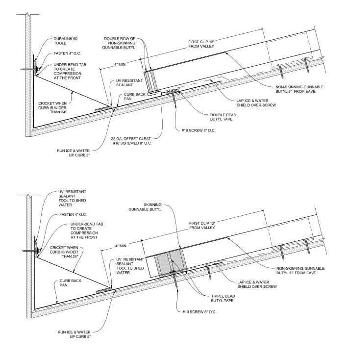
**Note:** All screws must be fastened into solid substrate. Flashing must be lapped 4" with 3 rows of gunnable sealant.
