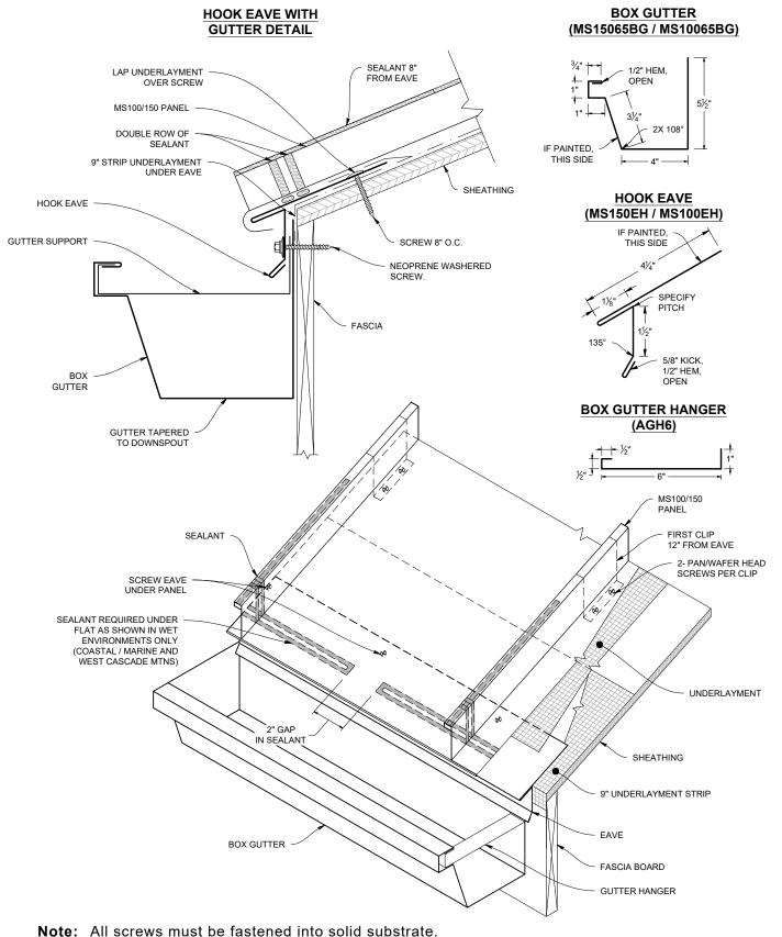
Flashing must be lapped 4" with 3 rows of gunnable sealant.
