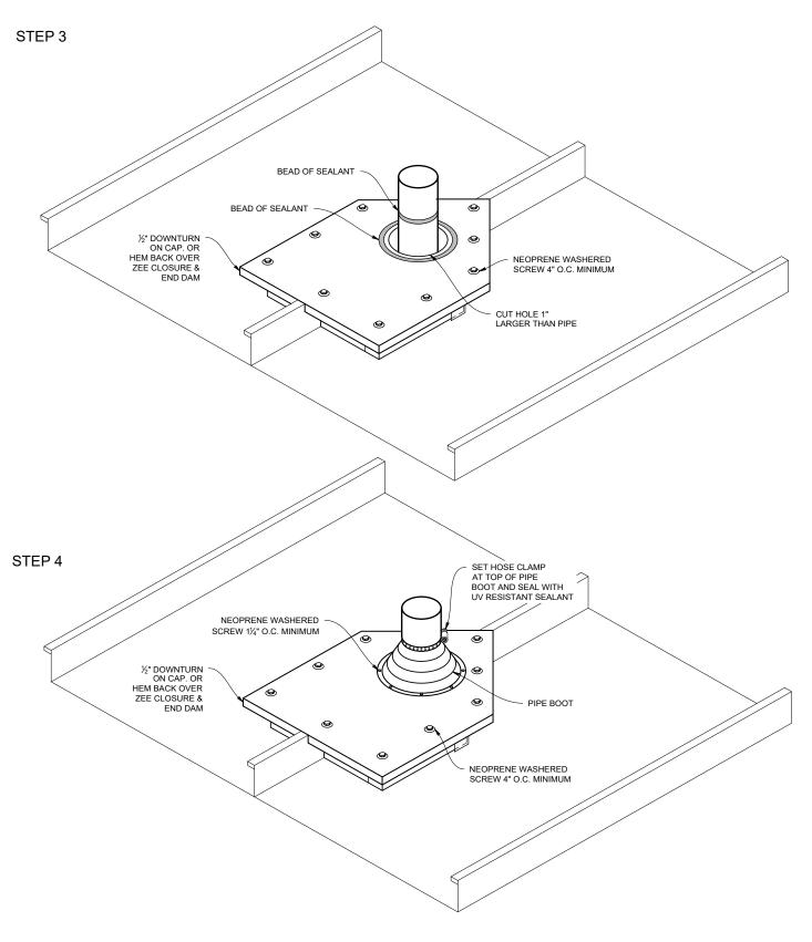
**Note:** All screws must be fastened into solid substrate. Flashing must be lapped 4" with 3 rows of gunnable sealant.
