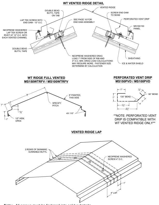
**Note:** All screws must be fastened into solid substrate. Flashing must be lapped 4" with 3 rows of gunnable sealant.
