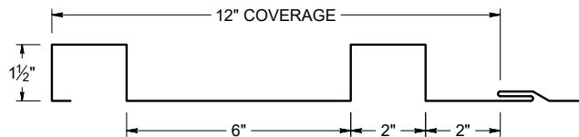
Screw Flange panels in this profile require additional material (drop/waste) and must be slit to a custom size. Inquire for custom pricing and availability.
