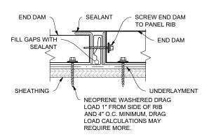
**Note:** All screws must be fastened into solid substrate. Flashing must be lapped 4" with 3 rows of gunnable butyl.
