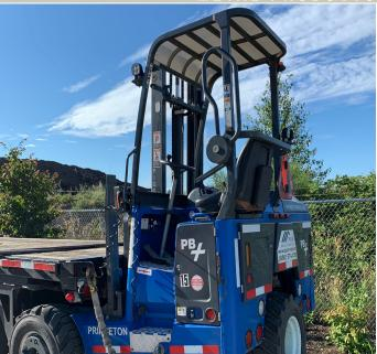
Mounted on the rear of our semitrailer, the trailer-mounted "piggy-back" forklift will accompany you right to your place of use, opening up unprecedented possibilities in terms of transportation. It can travel sideways, carrying panels up to 40' long, allowing delivery in locations that would typically be considered impossible to reach.
