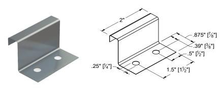
STANDARD CLIP: For UL rated non-engineered and solid deck applications
