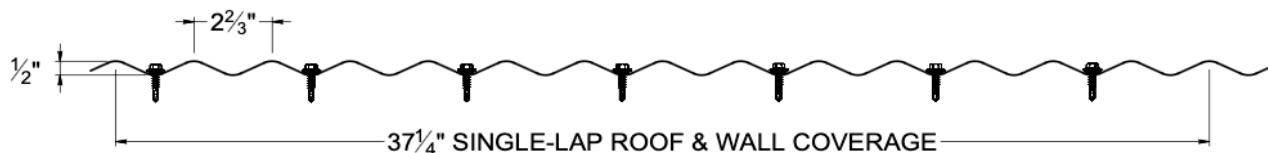
Roofing Panel Profile and Typical Installation
