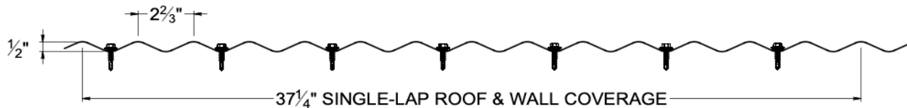
Roofing Panel Profile and Typical Installation
