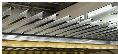
Purlin mill shown above before purlin is formed. Below are the purlins (zee).
